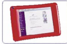
Fig. 1. B5-size workpanel from Höft&Wessel with an 8.2" DSTN-Display, 32bit/200 MHz CPU and four wireless communication channels (see also [1]).
